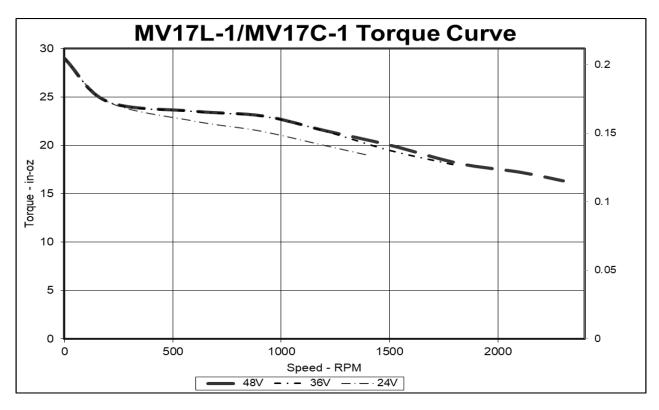
Torque curves represent motor torque at the specified voltage when the TQL command is set to "100%". These curves represent torque up to 100% duty cycle depending on ambient temperature, heat sinking and air flow.
