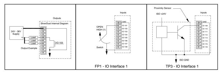
Sinking Output configuration ON or LOW = closed circuit OFF or HIGH = open circuit
