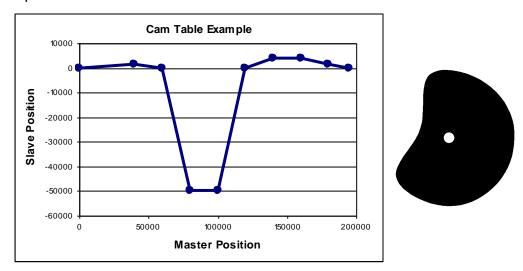
Above is the cam example used in this application note. A cam table, the corresponding graph of the cam data, and an image of the physical cam is provided.
